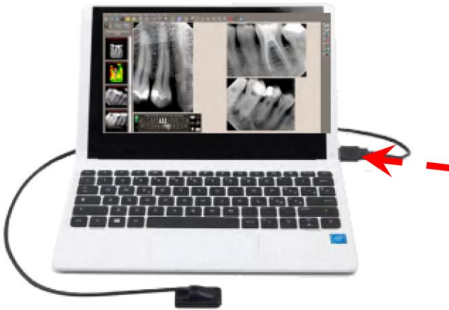
Connect the sensor to the USB® port of the PC (stand-alone sensor)
