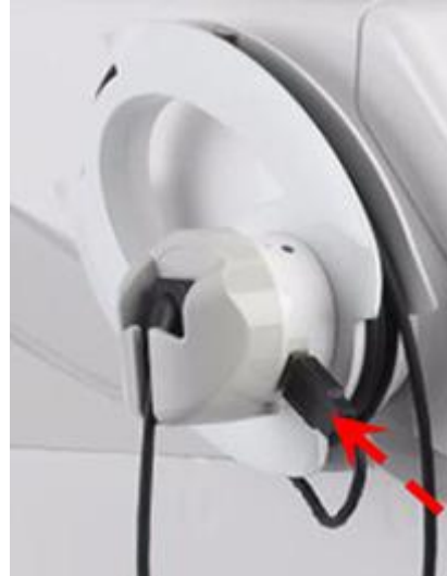
Connect the sensor to the interface integrated in the dental unit (sensor integrated in dental unit)
